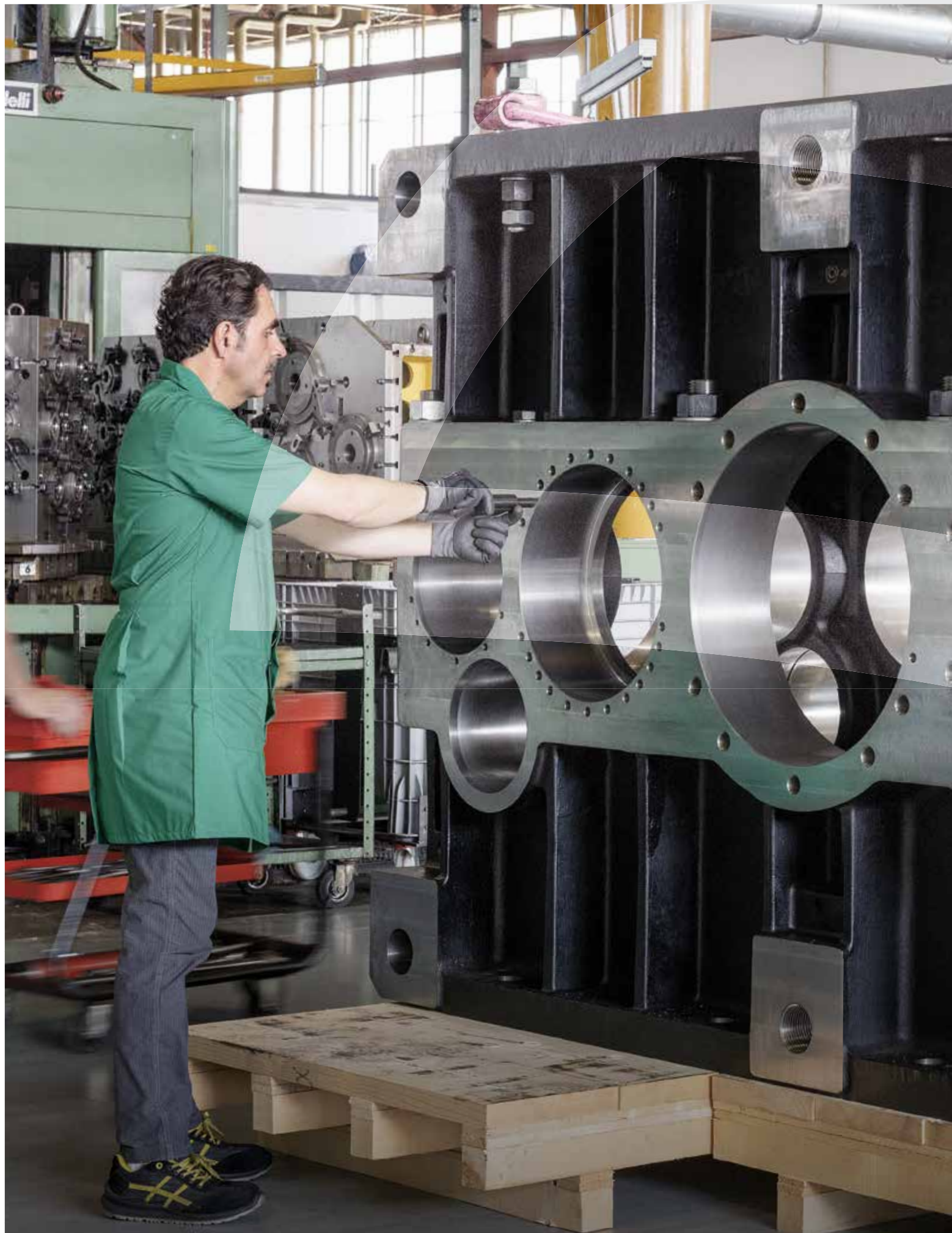
Dedicated area for extra-large housings equipped with boring, milling and 3D control system.
